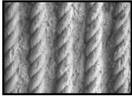
Fractured Rope Rib (2" OC rope) P/C 230715 0.090 mil Styrene P/C 230475 0.110 mil ABS
